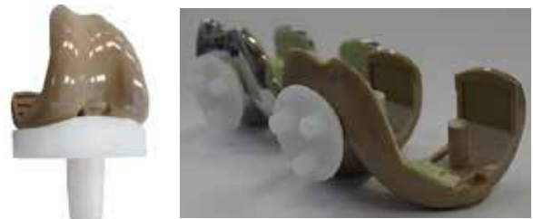
Figure 1: Images of the all-polymer total knee replacement. Left: the PEEK femoral component coupled with an all-polyethylene tibial component, right: the patellofemoral joint
