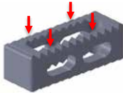
Figure 7 (a) Key failure points of the lumbar cages.
