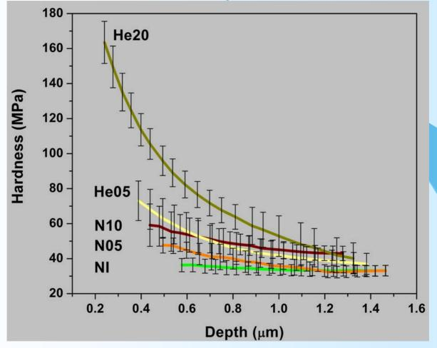
Helium implantation provided higher hardness The higher the fluence, the harder the surface
