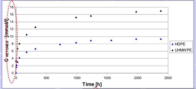
Ketone amount was estimated considering the IR absorption (1718 cm<sup>-1</sup>) in the spectral subtraction. Only ketones are reported because they are easily detectable, unlike hydroperoxides.
