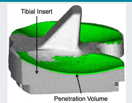
MicroCT – can provide analysis of wear and creep from retrievals; particularly useful for UHMWPE TKR components where radiographic assessment of wear is poor
