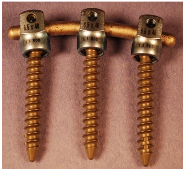
Figure 1: Retrieved implant consisting of three pedicle screws and titanium rod utilized in a spinal fusion. The screws are inserted into the pedicles of the vertebrae and join by the rod, restoring height to the spine segment. The retrieval was provided by the Implant Research Center at Drexel University.
