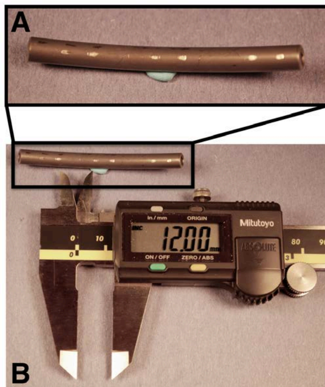
Figure 7: (A) Tri-level spinal fusion rod retrieval has clear notches indicating where the pedicle screws interface with the rod. The distance between notches (B) was measured as 12 mm. The height of the clip was designed to allow 1.5 mm of clearance on each side so the pedicle screws do not impinge on the clip.
