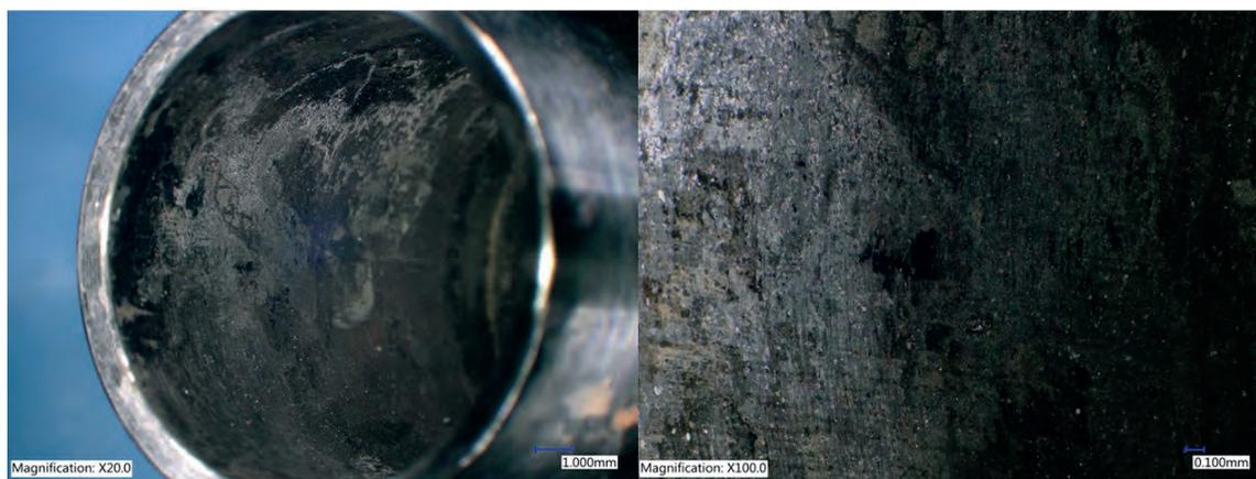
*Figure 21. Optical micrographs of sample CW-H0915, showing black deposits throughout the taper.*
