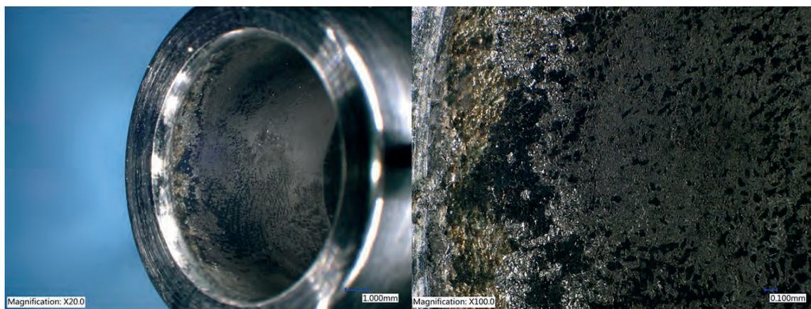
*Figure 27. Optical micrographs of sample RI-H0801, exhibiting proximal discoloration, black deposits and areas with a shiny appearance.*
