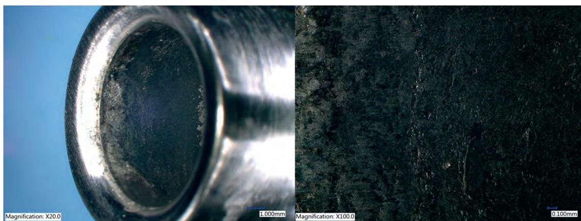
Figure 26. Optical micrographs of sample CW-H0201, with black deposits proximally and areas with a shiny appearance.
