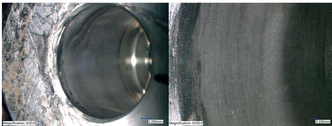
*Figure 28. Optical micrographs of sample SHB-H0689, with black deposits distally and a hazy appearance throughout the taper.*
