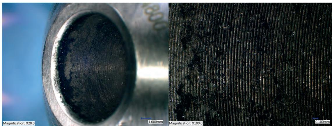
Figure 25. Optical micrographs of sample CW-H0616 exhibiting imprinting with black deposits.
