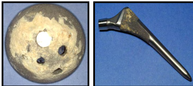
Figure 2-1: A retrieved porous tantalum acetabular shell (left) and femoral stem (right).
