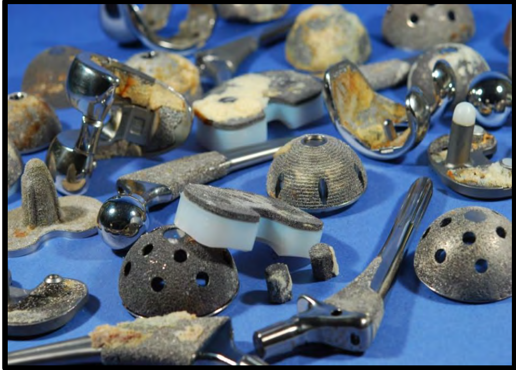
Figure 1-1: Representative sampling of retrieved cementless implants collected through the multicenter retrieval program. Image courtesy of Christina Arnholt.
