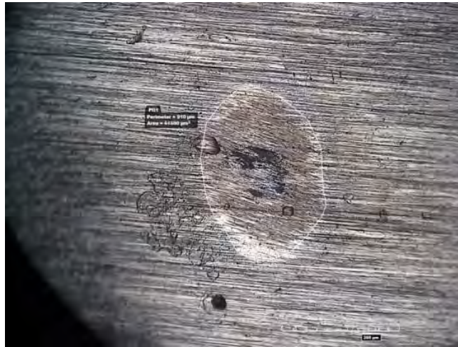
Figure 67: Pin tips and disks inspected using scanning electron microscopy (JEOL JSM-5600) and optical microscopy (KH-8700, HIROX) for quantification of contact area. Area calculation feature is available on the KH-8700 by selecting the worn area.
