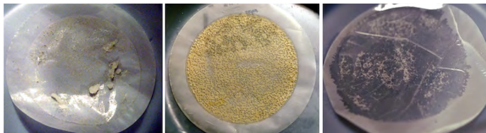
Figure 1-5. Representative images of formalin-fixed porcine tissue digests following vacuum filtration. Qualitatively, large residual tissue debris were not observed on membranes from tissues digested in 15.8M \text{HNO}_3 .
