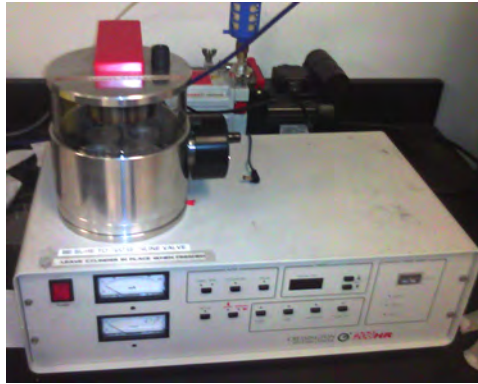
Figure 4-1. 208HR High Resolution Cressington Sputter Coater
