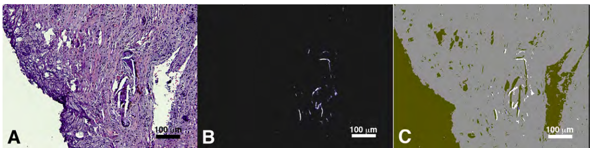
Figure 2-2. Polyethylene wear debris characterization in revised hip tissue. A: Brightfield image showing the tissue area, (B) polarized light image showing polyethylene particles, and (C) a composite of A and B generated as layers using customized threshold operations programmed in Matlab™ to determine the particle number per mm 2 area of tissue (100X).
