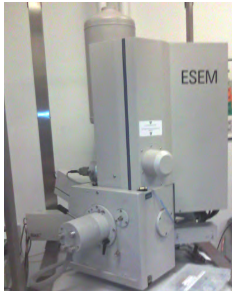
Figure 4-2. XL30 environmental scanning electron microscope (FEI/Phillips, Hillsboro, OR).
