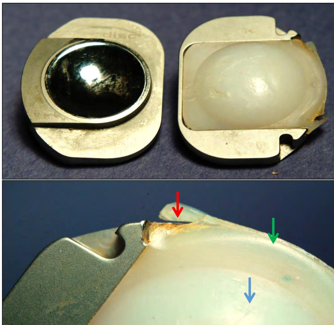
**Figure 3-5. Representative fixed-bearing L-TDR retrieval components (top). All fixed-bearing UHMWPE cores showed evidence of burnishing (green arrow) and mild abrasive scratching (blue arrow). Impingement was noted in two patients and the respective components evidenced plastic deformation (red arrow).**
