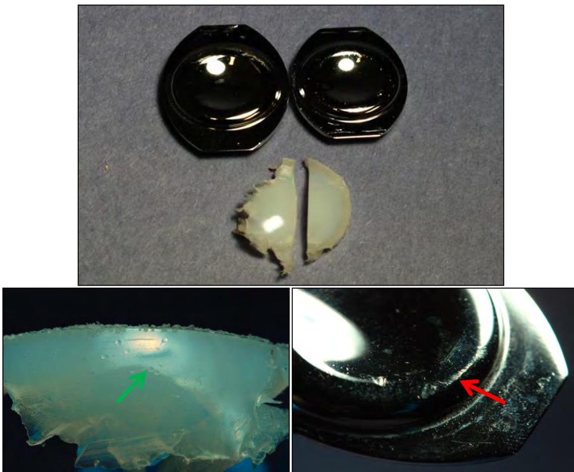
**Figure 3-7. Representative mobile-bearing L-TDR retrieval components (top). Two of four patients with mobile-bearing UHMWPE cores showed evidence of burnishing, pitting (green arrow). Minor unidirectional scratches were noted on endplates from all patients (red arrow).**
