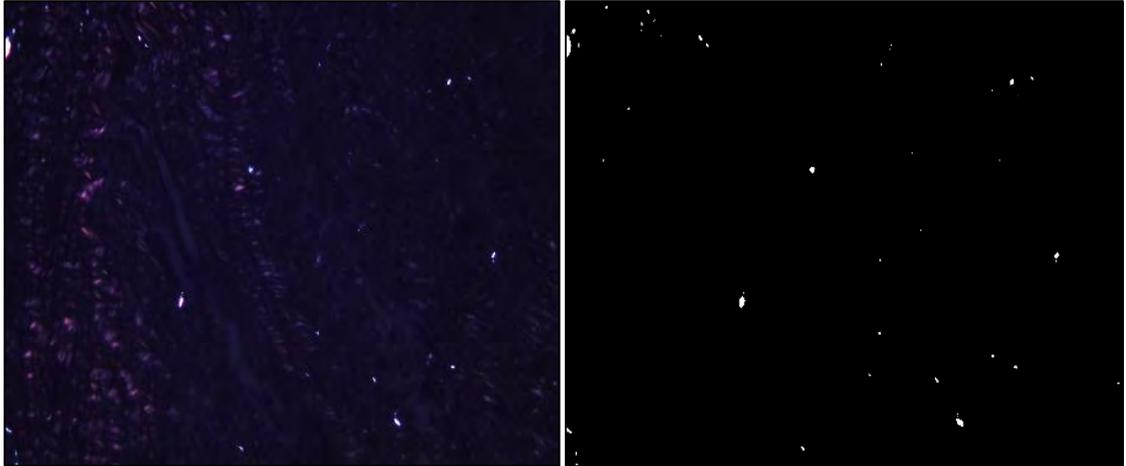
**Figure 3-3. Representative images of L-TDR periprosthetic tissues with wear particles under polarized light (left) followed by thresholding for UHMWPE particles in MATLAB (right).**
