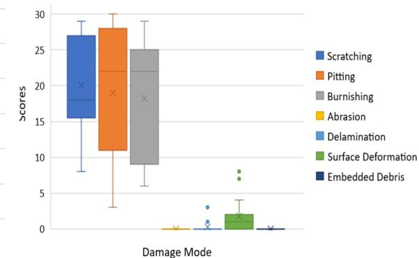
Figure 7. Damage scores for superior polyethylene surface
