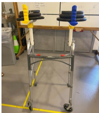
Added 55 lbs on each handlebar (total of 110 lbs on system)
