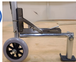
Detachable aluminum extension connected by hinge joint
