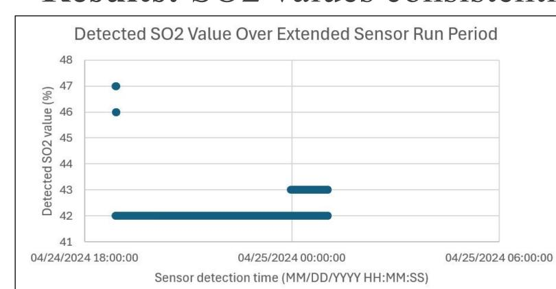
SO2 readings remained within 2% of 42% - TEST **PASSED**
