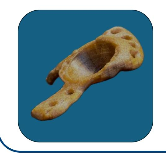
Temp. 400C Layer Height 0.15 mm Speed 25 mm/s Anneal 200C, 2hrs
