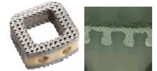
Fig 2. Spinal interbody utilizing PTSC (left) and detailed view of its PEEK/Titanium inter-digitation layer (right)
