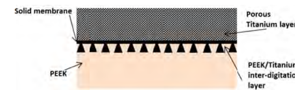
Fig 1. Schematic of PTSC four-layered structure
