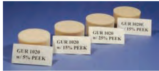
Figure 1: PEEK fiber reinforced GUR1020 resin HXLPE with 5, 15 and 25%/w PEEK fibers and GUR 1020E with 15%/w.
