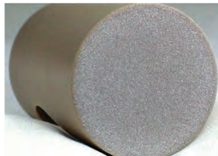
Hydroxyapatite plasma spray coating on PEEK with no adverse effects on the substrate
