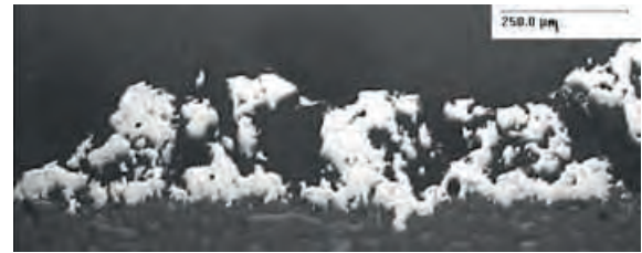
Fig. 2- Porous Ti-coating; micrographic cross-section
