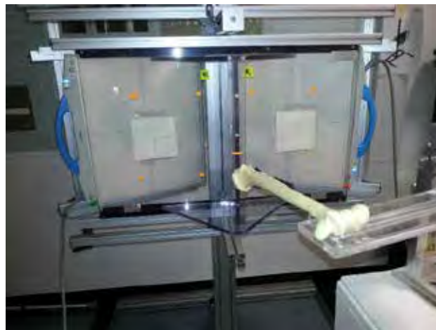
Figure 1. Bone model held in a horizontal position in the upright patient stereo imaging setup.
