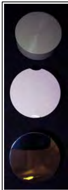
Figure 1: A representative disc from each counterface material: PEEK (top), Biolox TM ceramic (middle), and polished CoCr (bottom). The hemispherical indentations on the ceramic disc were part of the fixation mechanism to hold the disc in the test basin; they were located far from the area of articulation so they should not have affected the wear of the UHMWPE pins. Note that machining marks can still be seen on the PEEK disc – the material was tested as-machined; the other two discs had highly polished surfaces.
