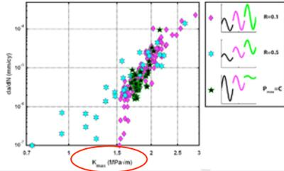
Implication: stable crack growth can occur in the absence of cyclic loading - creep/brittle behavior
