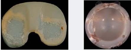
Embrittled subsurface layer has poor crack resistance
