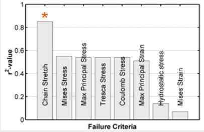
The chain stretch failure model is significantly better than other failure models for UHMWPE Bergström, Rimnac, Kurtz JOR, 2005
