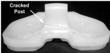
In vitro fracture under cyclic loading
