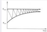
\*FCP tests of UHMWPE primarily conducted in this manner
