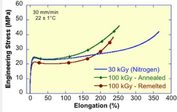
Reduced ductility (annealed and remelted);
