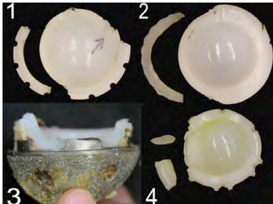
Figure 1. Fractures in four crosslinked UHMWPE acetabular cups that all have elevated rim designs [4].
